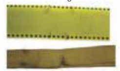
Discoloration and brittle or Stiff area due to Chemical or Ultraviolet sunlight damage
