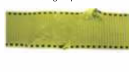
Broken or Worn Stitches in Load Bearing Spliced Area
